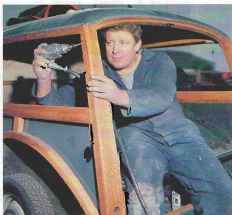
Restoring the woodwork on a Traveller
