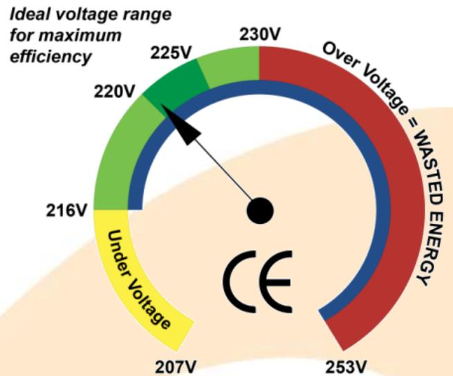
Equipment carrying the CE mark must be capable of operating between 207-253V.
