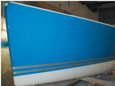
Composite hull: cedar strips planks scarfed together, then faired, sheathed in carbon fibre, smoothed to a fine finish with epoxy coatings and finished with Awlgrip paint.
